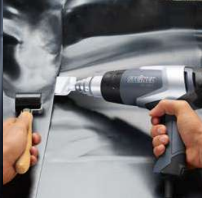
▲ Welding pond liner HG 2320 E
