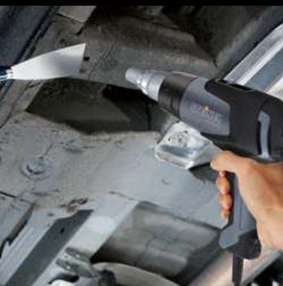
▼ Removing underseal HG 2120 E
