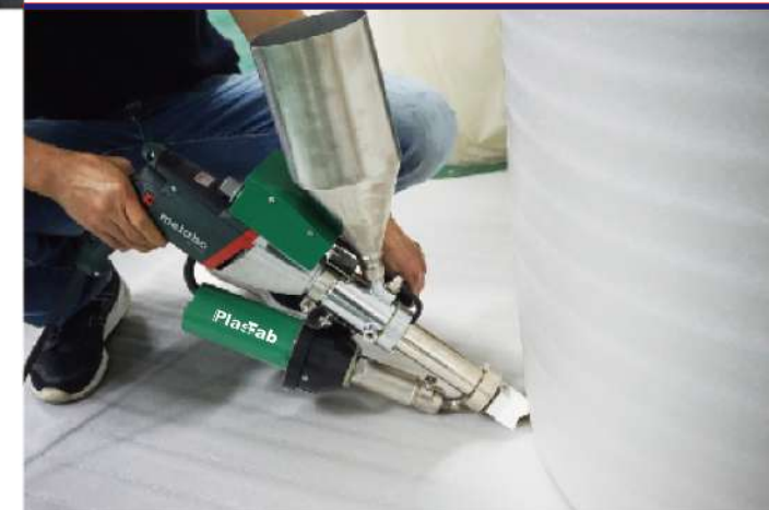
Plastic Tank Welding PFE620
